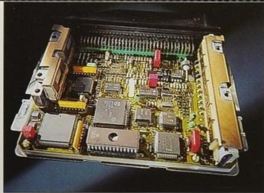
The BMW Digital Motor Electronics (DME) are among the most sophisticated and reliable open-chain and closed-loop systems
